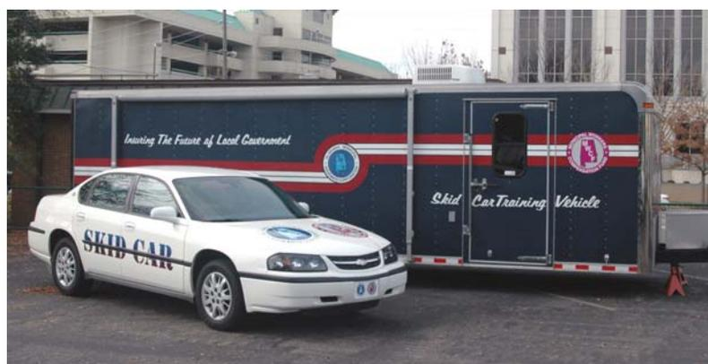
The Skidcar System is an advanced, computer-controlled driver training tool. Its ladder frame consists of hydraulic outrigger casters mounted to the suspension of the training vehicle. When activated by the instructor, the System lifts the vehicle off the ground just enough to compromise the tire adhesion to the road surface. As a result, the car skids as if it were going 60 miles per hour, when in reality it is traveling at a much safer speed (6 to 25 m.p.h.).
